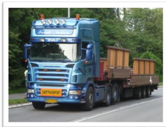
Photo 5 Transport of bridge sections
